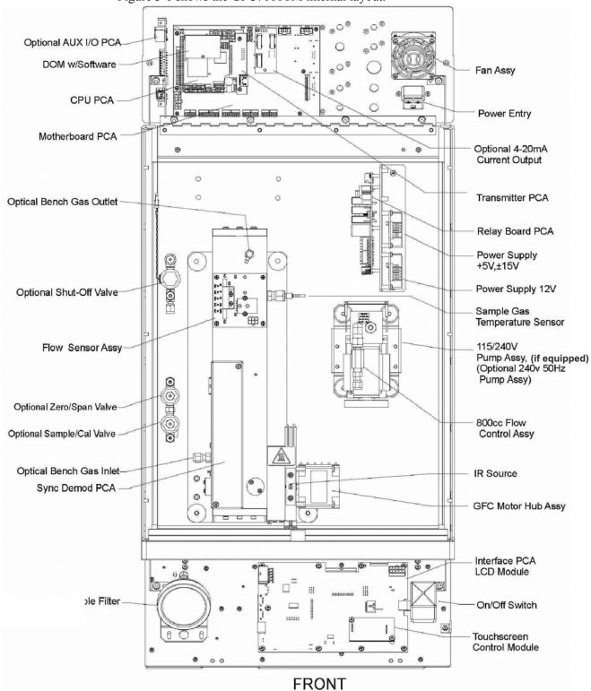
Figure 3-6 shows the GFC7001TM internal layout.
